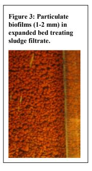
Our technology is a method of process intensification that is based on the natural immobilization of microbes, which grow as biofilms on small particles of glassy coke (Fig. 2) that are retained in the bioreactor. These bioparticles (Fig. 3) provide 1,800 m<sup>2</sup> of superficial surface area per m<sup>3</sup> of expanded bed and it is this huge surface area of active biofilm that lies at the heart of our highly effective bioprocess technology.
